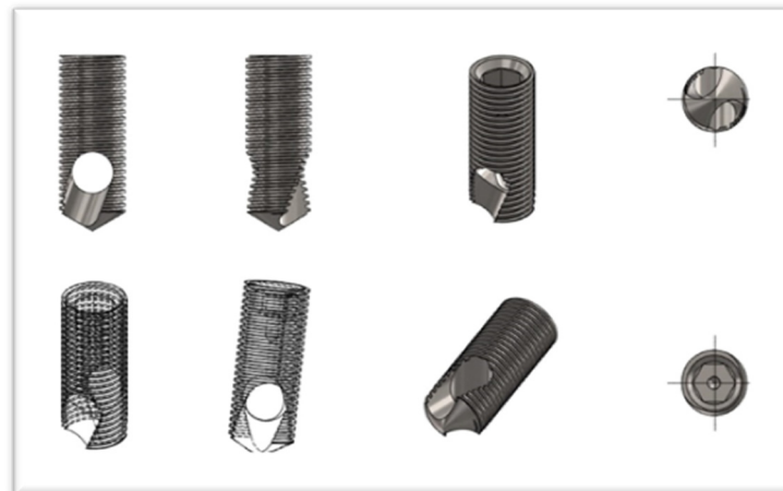
Figure 1. New biomechanical screw (BKS) of 4 mm width and 10 mm length.
